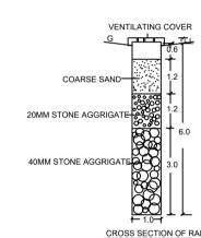
CROSS SECTION OF RAIN WATER HARVESTING WELL
